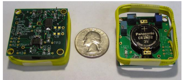
Figure 1. Both sides of operational SNUPI sensor nodes
